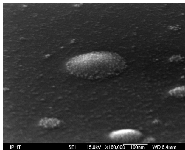
Fig. 4. Distribution of nanoparticles after surface adsorption of product suspension from styrene polymerization in presence of lipophilized gold nanoparticles; ensembles of gold nanoparticles embedded in a organic matrix at silicon chip surface; SEM image.
